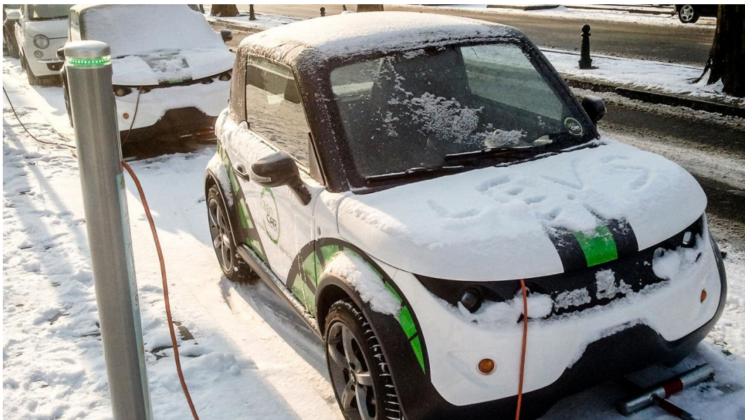
Figure 11: Your EV battery doesn't like extreme weather any more than you do, but plugging in can allow the EV thermal management systems to help keep the battery comfortable.
