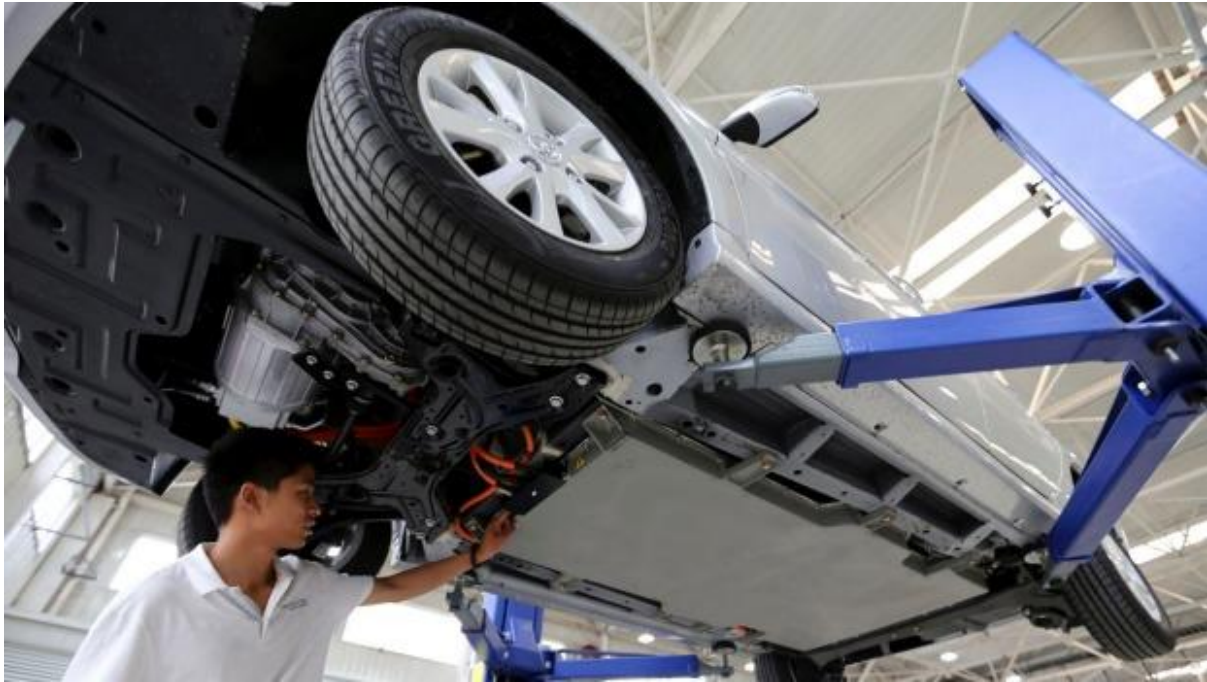
Figure 13: An authorised technician uses an industrial hoist to help inspect the high-voltage underfloor battery in an electric vehicle. Do not try this at home!
