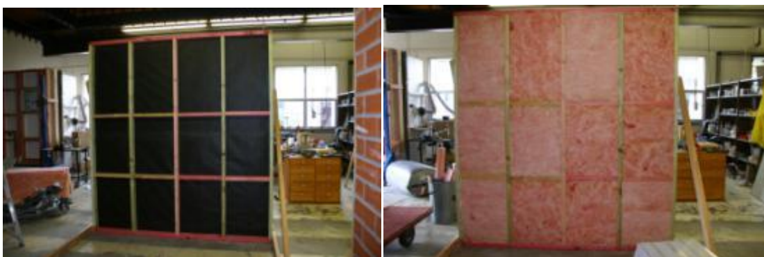
Figure 19 & 20: Frame before insulation (D4862) and with well fitted R 2.8 glasswool insulation (D4862a)
