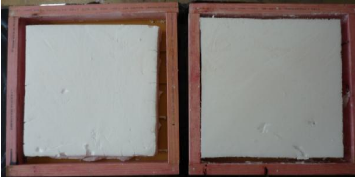
Figure 27: Shrinkage in low wall specimen C1E (left) after aging following ‘AS 4073-1993 Appendix H’ compared to control specimen C1A
