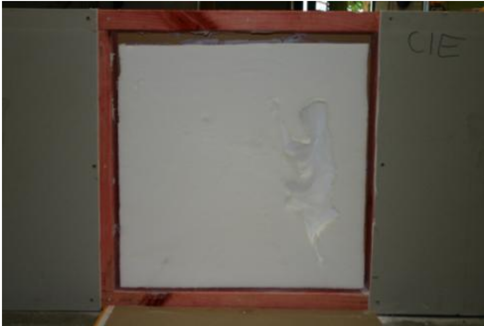
Figure 24: : Shrinkage in low wall C1, specimen C1D.
