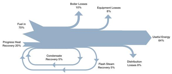
Figure 4: Steam System Energy Balance "Good" System Efficiency
