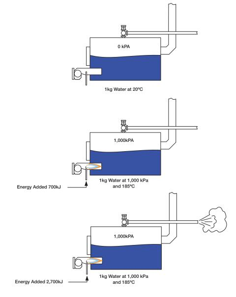
Figure 9: Steam Generation under Pressure
