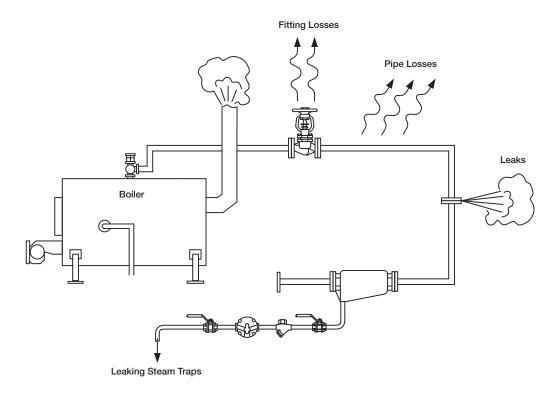
Figure 6: Distribution System Losses
