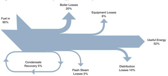
Figure 3 shows the efficiency of a typical steam system.
