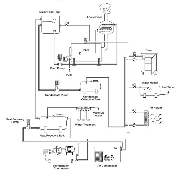
Figure 1: Outline Diagram of a Typical Steam System
