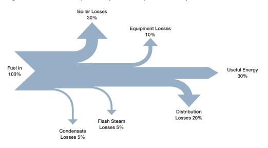
Figure 2 shows an example of a system with poor efficiency.
