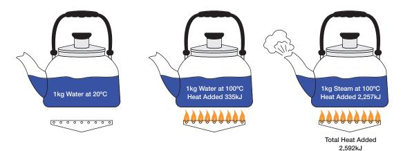
Figure 8: Steam Generation at Atmospheric Pressure
