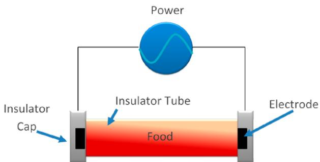
Direct resistance heating in an Ohmic Oven used to sterilise or cook food in a process line.
