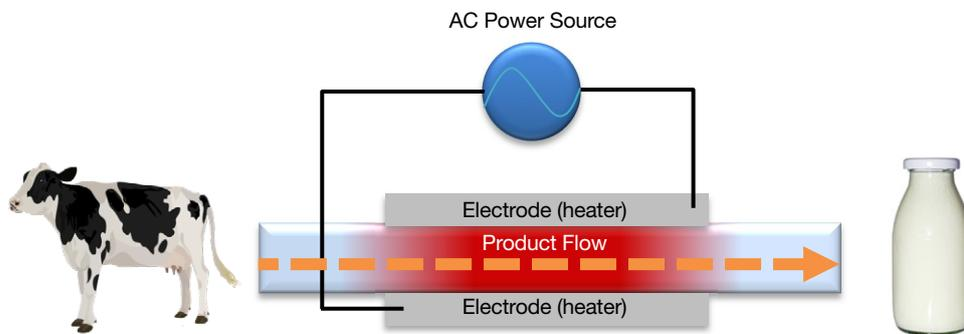
Figure 5. Controllable product flow rate through an ohmic heater. As used in pasteurisation and sterilisation.
