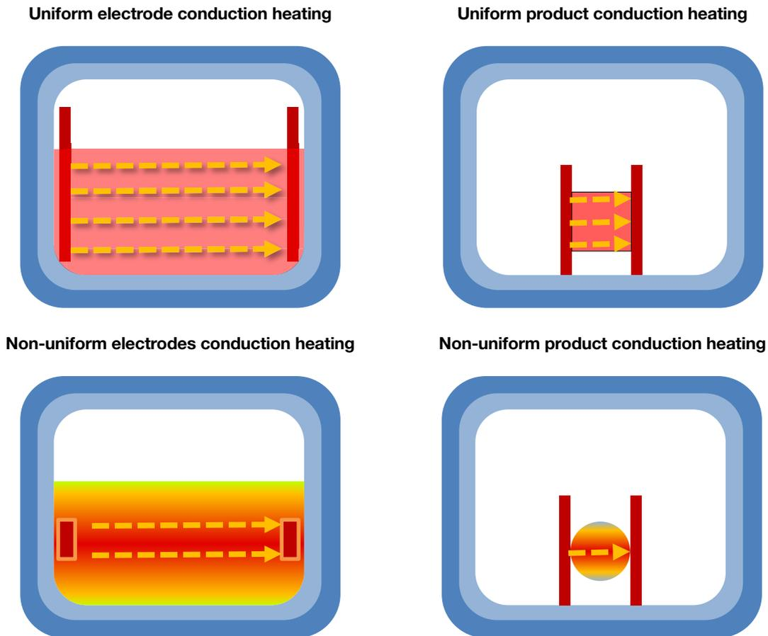
**Figure 4** Uniformity of heat transfer in different direct heating methods
