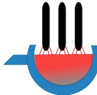
Direct resistance heating in an electric arc furnace used to melt and hold metal
