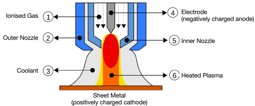
**Figure 8. Basic plasma cutter operation**
